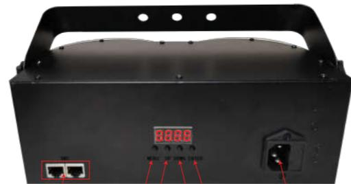
DMX input and output Function selection button Mode up selection key Mode down selection key Function confirmation button 220V power input
